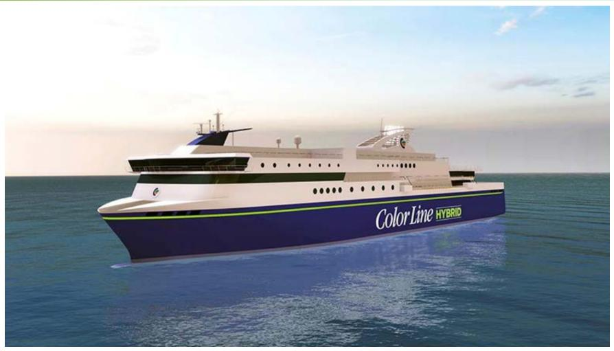
Hybrid propulsion system, 5 MWh battery system In operation from 2019, to be built by Kleven yard System integration by Siemens
