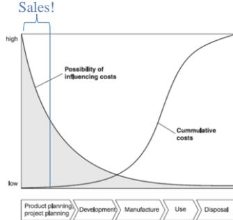
Fig. 2.2-2. Possibilities of influencing and establishing costs over the lifecycle of a product: The "dilemma of product development" (an example of a new design)
