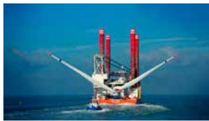
Three major exports from Norway to the offshore wind sector in 2013: The Aibel's HVDC platform (left, photo: Øyvind Sætre) in final construction phase before being towed to Germany), Nexans submarine power cables (middle, photo: Nexans), and a Fred Olsen installation of wind turbines (right, photo: Fred Olsen Wind Carrier).
