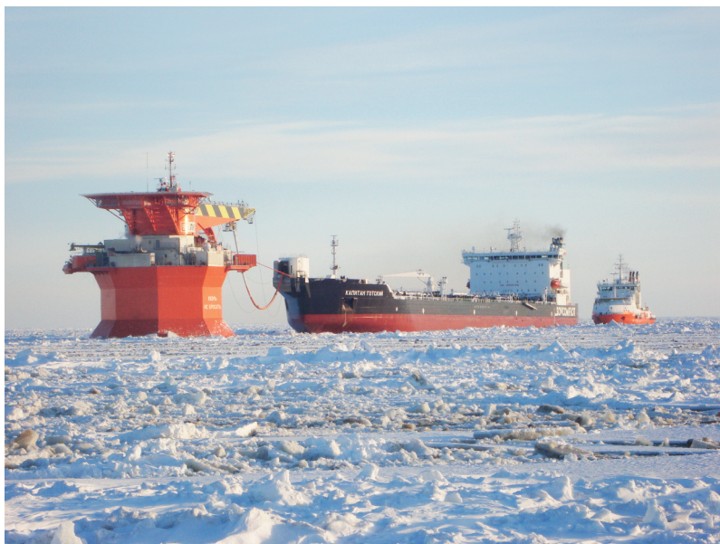
Fig. 5. A tanker loading at the Lukoil Varandey terminal with a stand by icebreaker astern of the tanker (photo Captain Gregory Martyuk).
